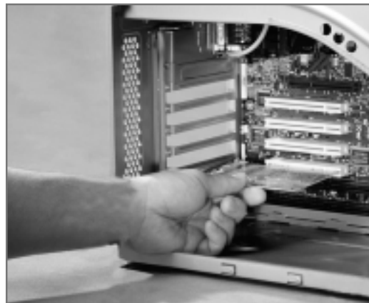
Figure 1 Installing the Adapter Card into a PCI Slot
